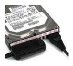
4. Plug the power adapter to power source and turn on the power . (Please make sure the voltage is between 100~240V)
